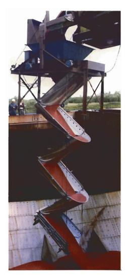
Our new "soft-drop" system is shown in operation in the photograph above. This system, which was developed by our engineering personnel in conjunction with Fraser Ship Repairs, minimizes product degradation by breaking the fall through a system of retractable chutes and reduces dusting thereby contributing to a cleaner environment and a safer and healthier work place.
