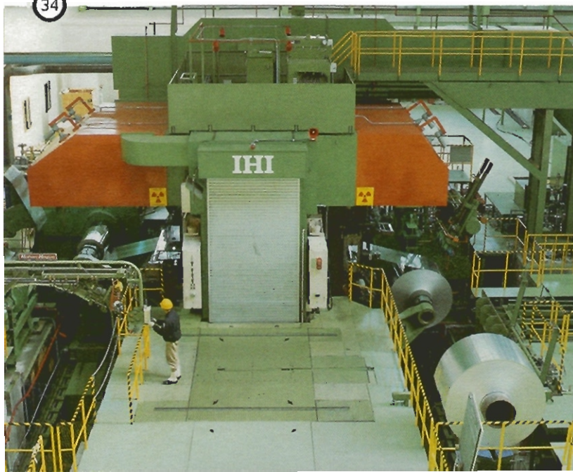
The growing market for aluminum rolled products will be served by Alcan Taihan Aluminum Limited in South Korea, using modern facilities such as this four-high, non-reversing cold rolling mill.
