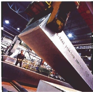
Large aluminum ingots are produced at Alcan's casting facilities at Grande-Baie (photo above) and Laterrière in Quebec and at Kitimat in British Columbia for shipment to various rolling mills in North America, Europe and the Asia/Pacific region.
