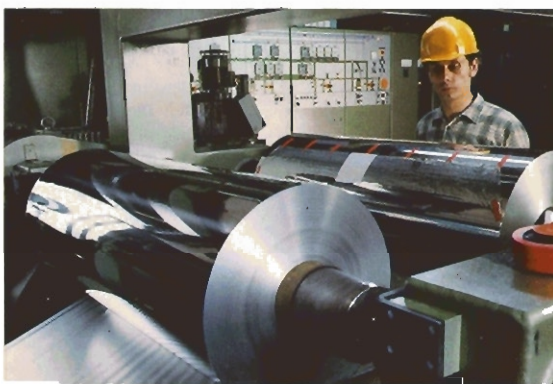
Bottom right: In Germany, Peter Meyer checks the flying splice on Ludenschaid's foil lacquering/laminating line. Coils can be changed without stopping production, a major aid to productivity.
