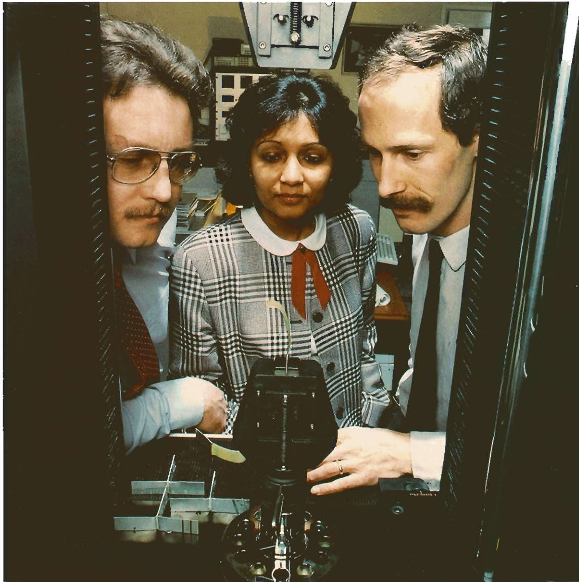
Dr. Richard Dickson, Dr. Rowena Landham and Bill Marwick, senior scientists at the Banbury Laboratories in the U.K., use slow peel testing to examine adhesively-bonded joints, part of the aluminum structured vehicle technology research program.
