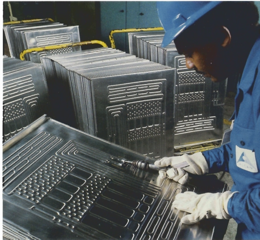
In Pindamonhangaba, Brazil, operator José Jacó Cesar prepares the tubing connections on a Roll-bond heat-exchanger panel. Roll-bond technology is used in a variety of applications from refrigerators to solar panels.
