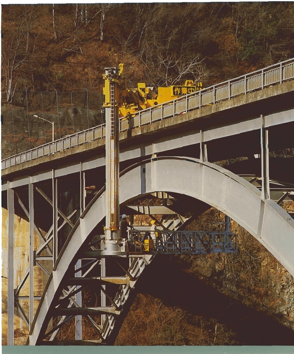
■ Alcan related company Nippon Light Metal Company, Ltd. developed this unique truck mounted bridge inspection equipment in cooperation with Japan's Ministry of Construction. The versatile equipment features a lightweight vertical boom and telescopic platform, both made of aluminum.
