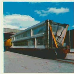
■ Aluminum rail cars, developed through a joint venture between Alcan and Thrall Manufacturing Company in the United States, are scheduled to go into service soon, having met Association of American Railroads standards in 1985.
