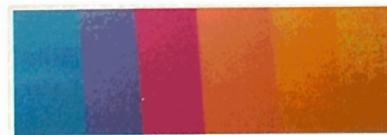
Aluminum surfaces can be treated by Alcan's interference colour anodizing process, to give the subtle shades in the colour spectrum above.
