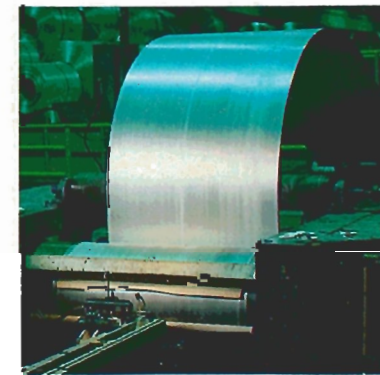
The continuous roll-caster takes molten metal directly from the furnace and solidifies it into aluminum sheet. This technology, which has been adopted for the new Malaysian sheet mill, provides the production flexibility required to meet the multiple variety of small orders typical of developing countries.
