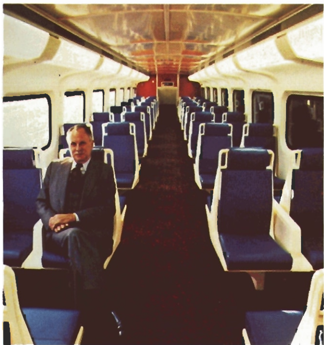
Canada—Bi-level commuter cars used by GO Transit, the Government of Ontario's rail transportation authority serving the Toronto area, derive their lightness from internal and external use of aluminum extrusions and sheet supplied by Alcan Canada Products Limited. E.J. White is chief executive officer and president of Hawker Siddeley Canada Ltd, the company that designed and built the new units.
