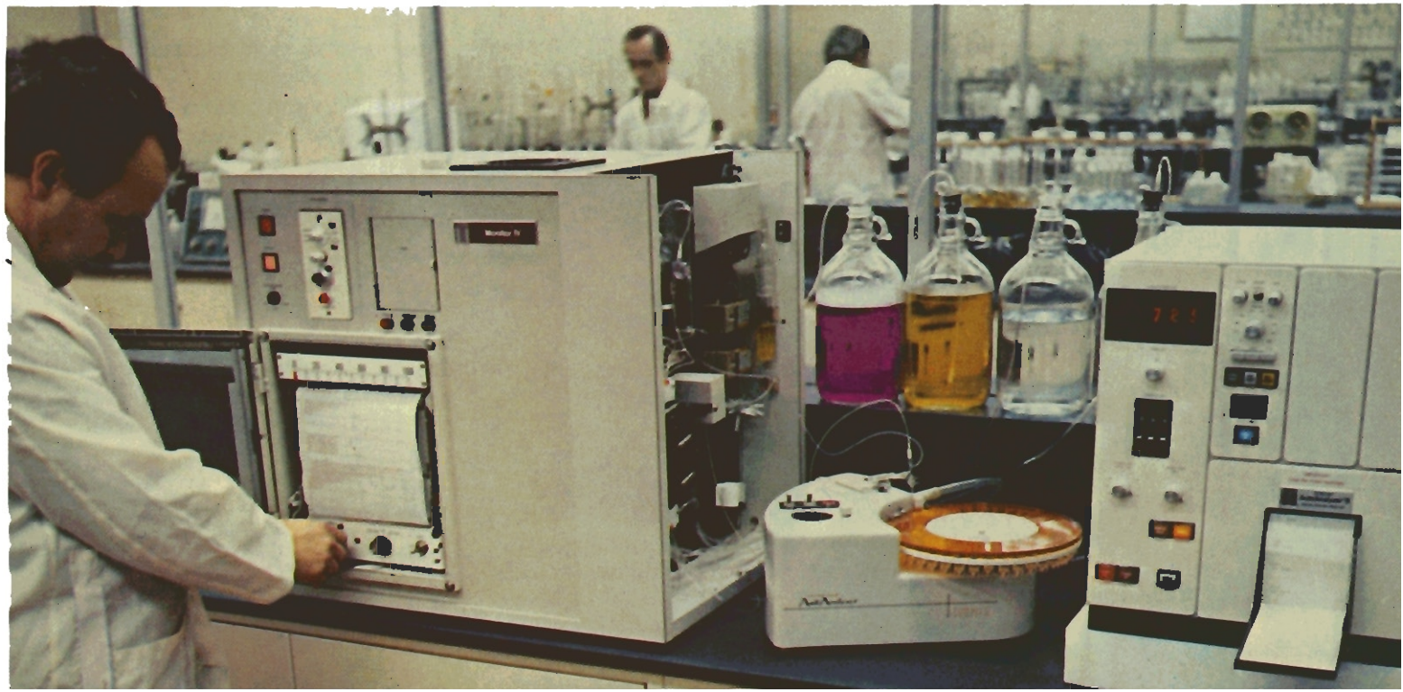
Below: Modular autoanalyzer system at Arvida automatically performs continuous chemical analysis and will be used to monitor and control chemical plant processes.
