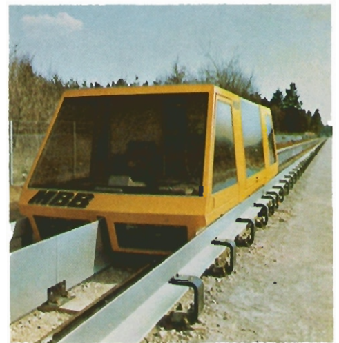
Experimental aluminum car for rapid transit in Germany uses magnetic field technology and linear motor propulsion.
