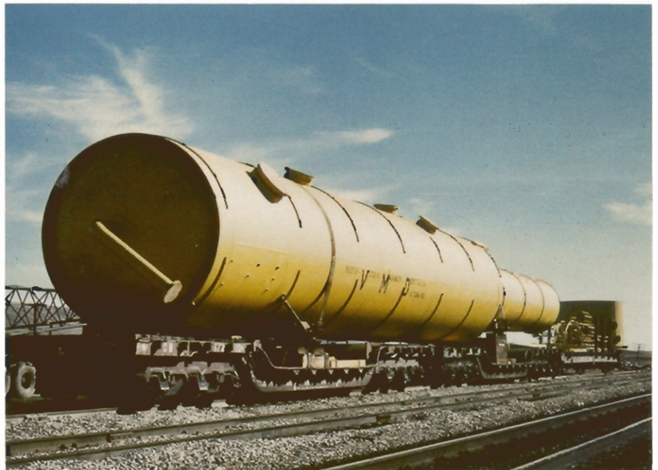
De-ethanizer process tower as seen on the railway siding upon its arrival near the plant site. The tower is 132 feet in length, 13 feet in diameter and weighs 185 tons.
