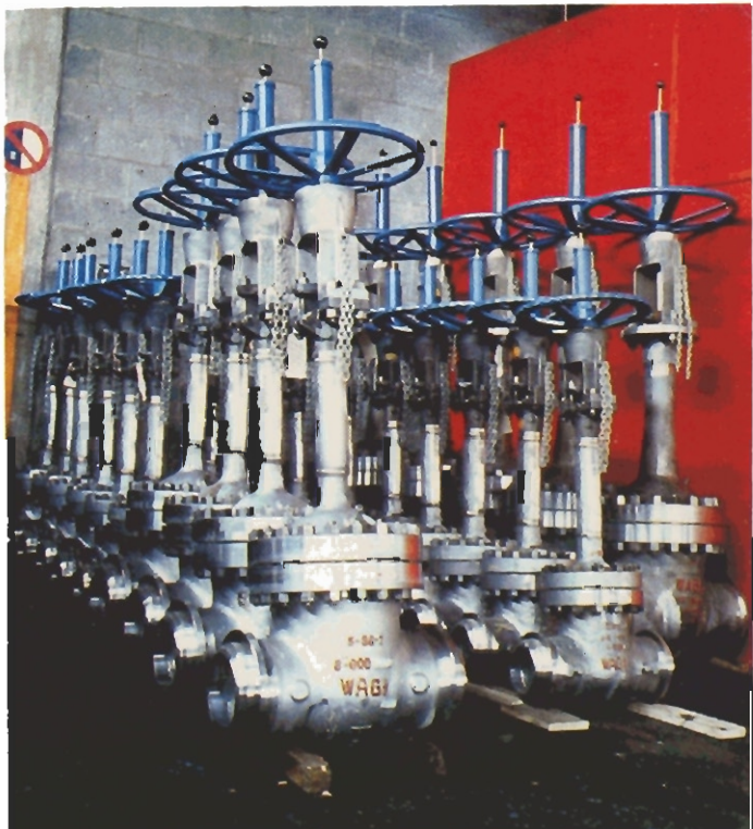
219.1 mm (8-inch) cryogenic gate valves, Ospiate, Milan Works, Italy
