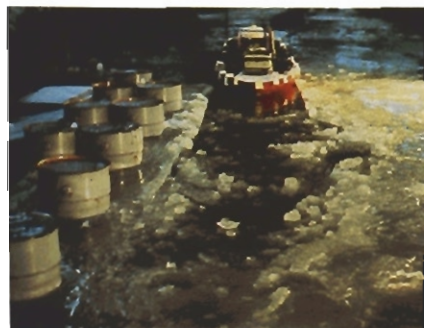
Ice-breaker tanker, model studies in simulated rafted ice.
