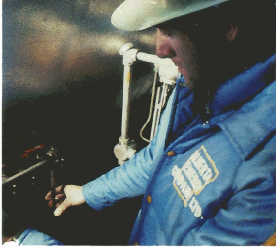
A small quantity of heavy oil is drawn off at the testing system sampling point.
