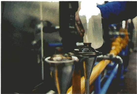
A solvent is employed to reduce the viscosity or heaviness of the oil.
