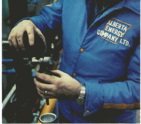
The oil is transferred to a laboratory measuring container suitable for use with a centrifuge.
