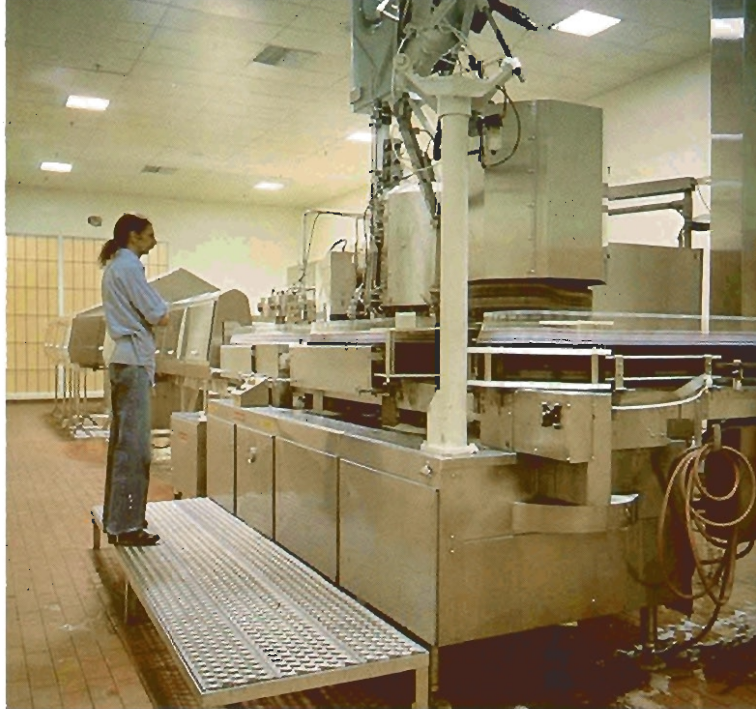
Operator Phil Pitts observes high speed bottle line in Blue Label Beverages' new Calgary plant as it fills soft-drink bottles at a rate up to 500 bottles per minute
