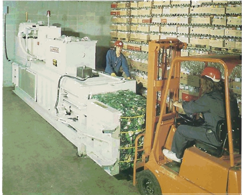
Contain-A-Way's plastic bailer crushes 7000 plastic bottles to produce a 700 pound bale which is shipped to South Carolina for recycling.
