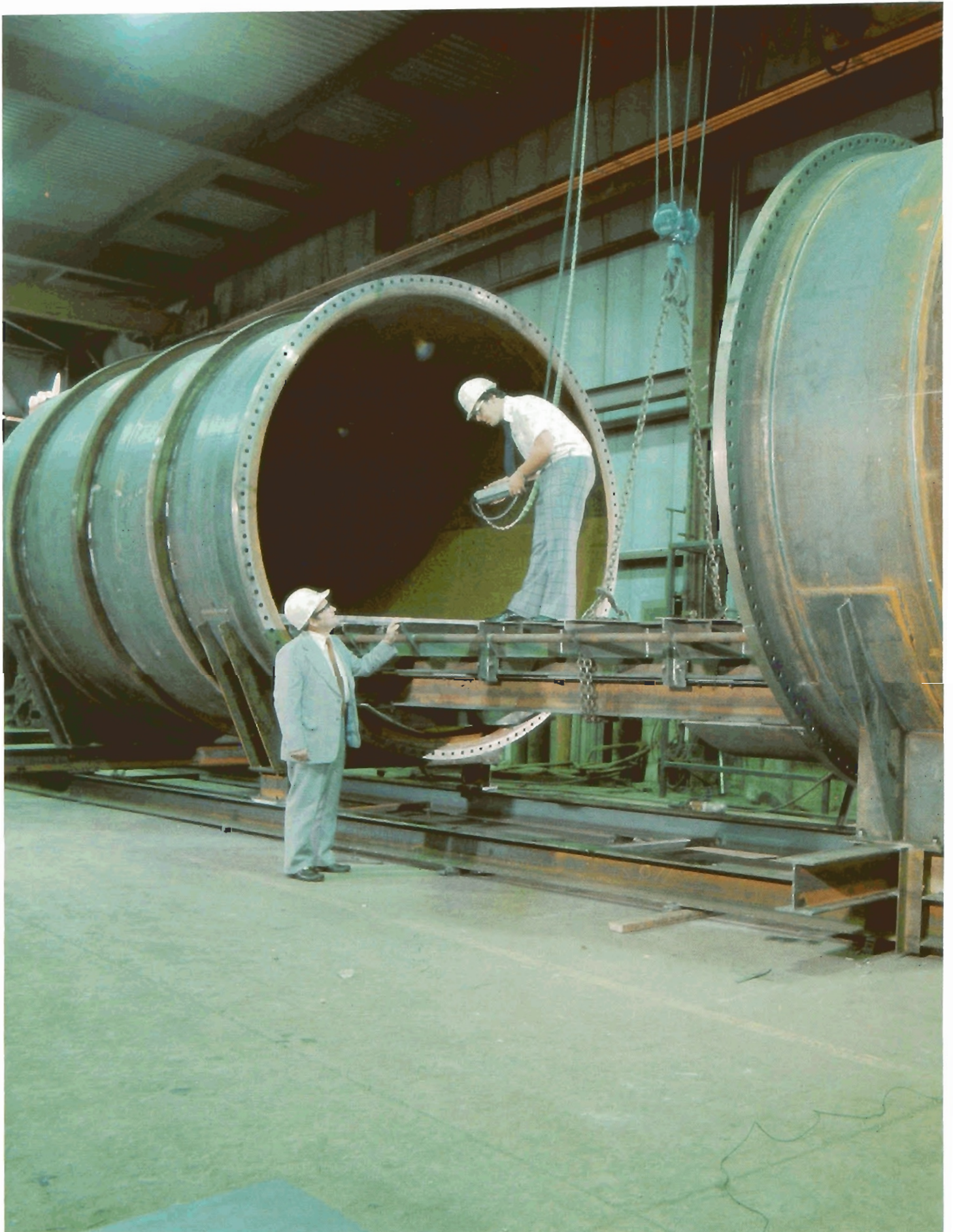
Fabrication of Cambrian's patented "CAMPRO" edible oil deodorizer recently sold to Best Foods Division of CPC International Inc. (producers of Mazola Oil) is well advanced
