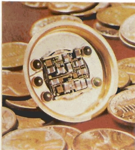
◀ Miniaturization in Communications by Cable TV is Shown in this Small Hybrid Thin-Film Amplifier Which is Almost as Small as a Penny
