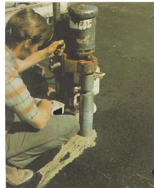
Povement Core Tests for City of Calgary, Conducted By Torchinsky Consulting Ltd.
