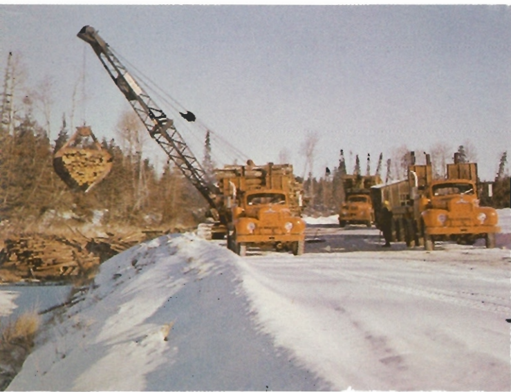
Truckloads of pulpwood arrive at a frozen river at which point a waiting crane unloads it onto the ice surface where it remains until the spring river drive begins.
