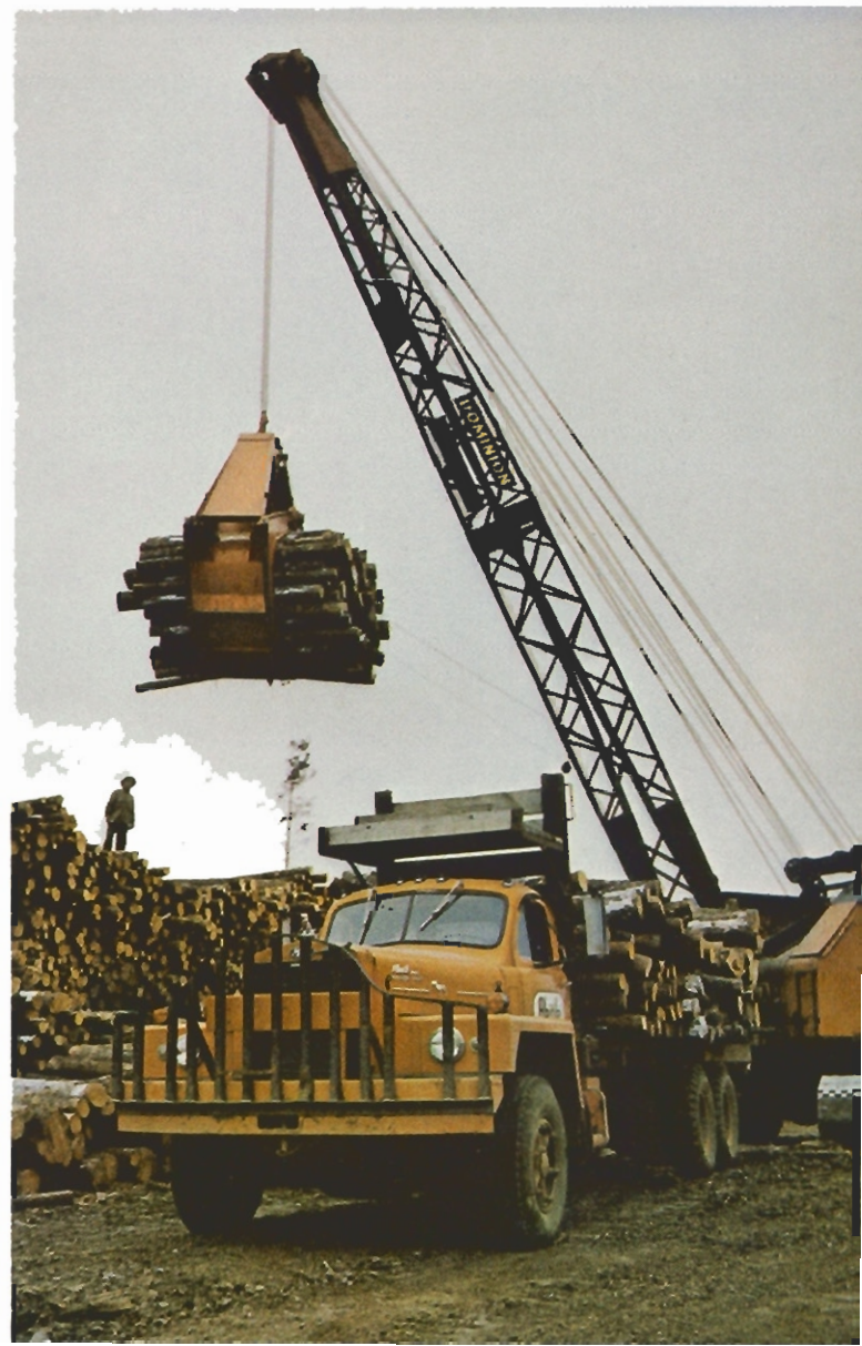
The versatile crane has many uses in our woods operations. In this scene it is loading eight foot wood at a transfer point for direct haul to the paper mill.
