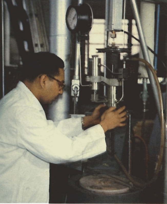
Chemical Engineer Shafi Hossain prepares an autoclave for the treatment of material at extremely high temperature and pressure. This is only one of the complex testing machines required by this laboratory to make certain that each of Abitibi's products is of the highest quality.
