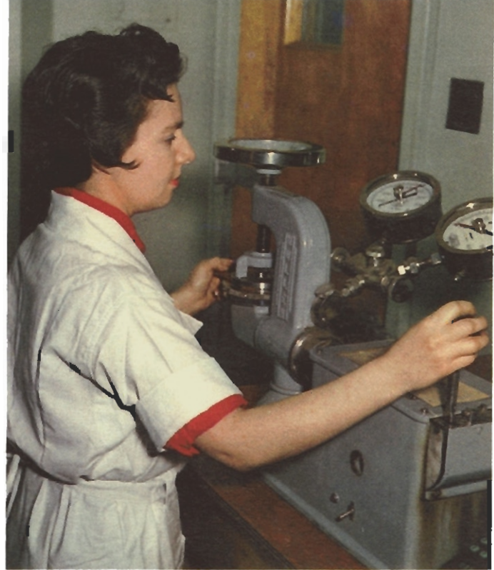
Abitibi Hardboard, as are all of the Company's many products, is subjected to rigorous quality control tests. One of these, in process here under the guidance of Virginia I. Willoughby, is the mullen, or burst, test designed to obtain a reading of our Hardboard's resistance to this type of rupture.
