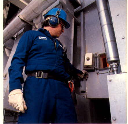
Tom Handyside wears protective equipment when checking burners in the hydrogen reforming heater of the new hydrocracker complex.
