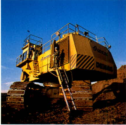
This equipment used to remove overburden at the oil sands plant receives 8 to 12 hours of preventive maintenance every week to ensure safe operation.
