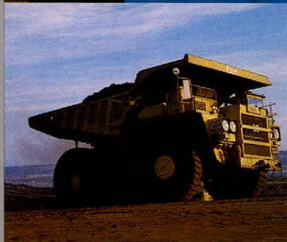
Rae Stephenson operates a 170-ton truck hauling overburden for dike construction.
