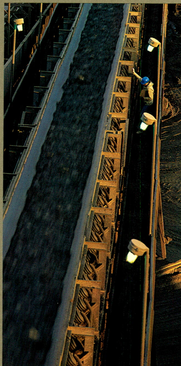
A superintendent inspects the conveyor belt carrying oil sands to the extraction unit.
