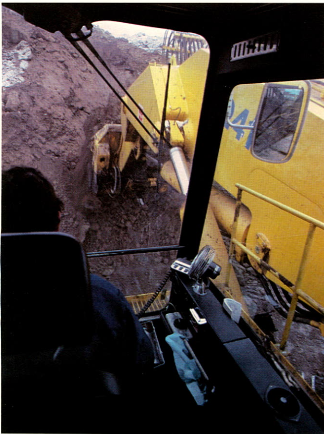
This new hydraulic shovel which commenced operation in 1980 added to overburden removal capacity at the oil sands plant. Overburden is removed to expose oil-bearing sands for mining.
