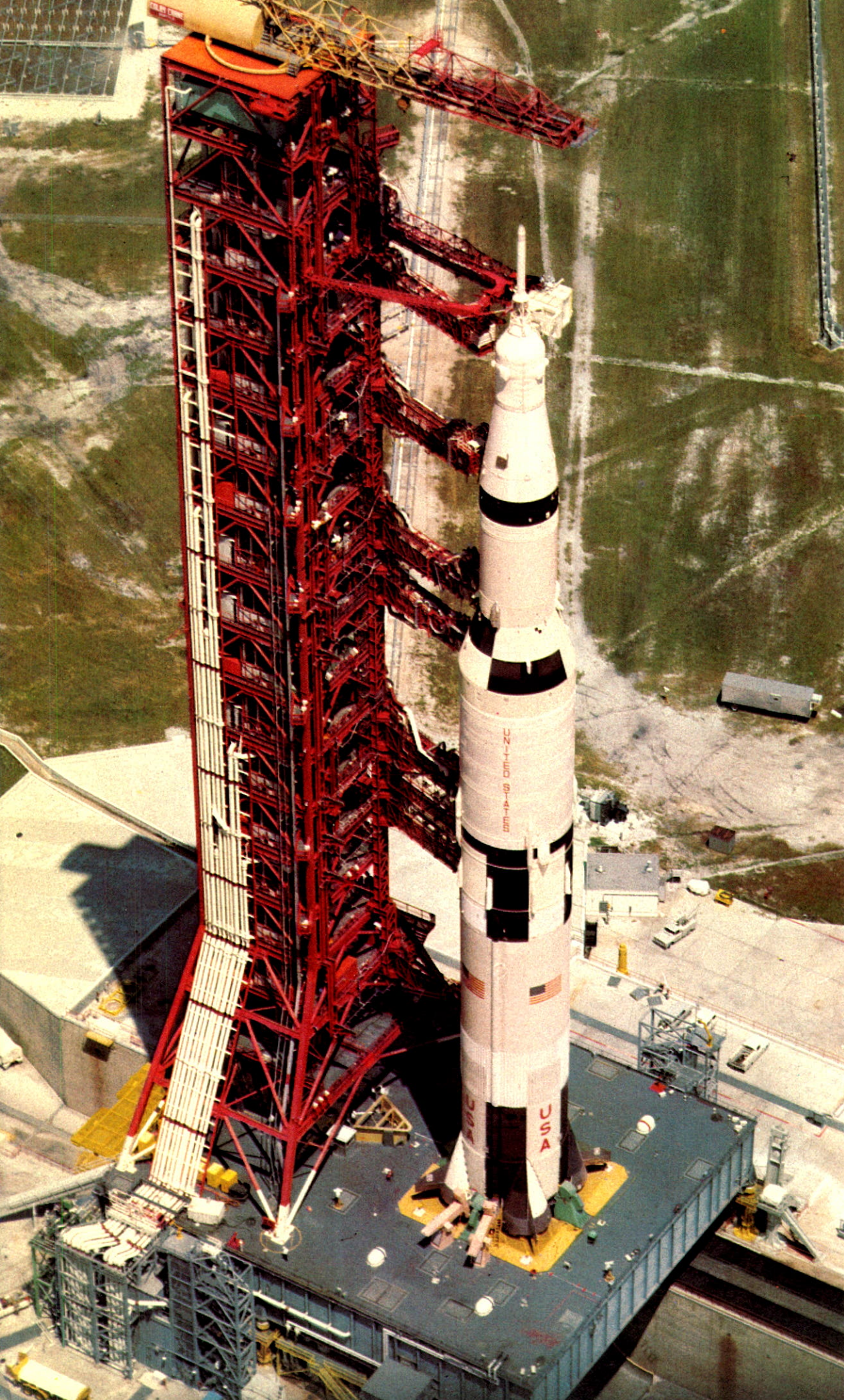
36-story Saturn V launch vehicle is scheduled for early flight with Apollo spacecraft as payload.
