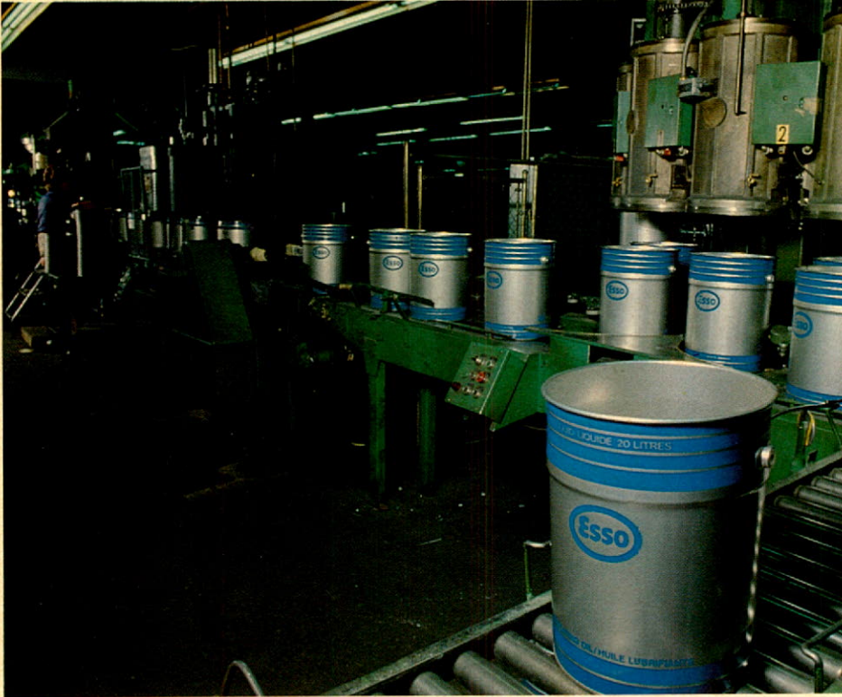
High speed air pressure tester, Container Division.
