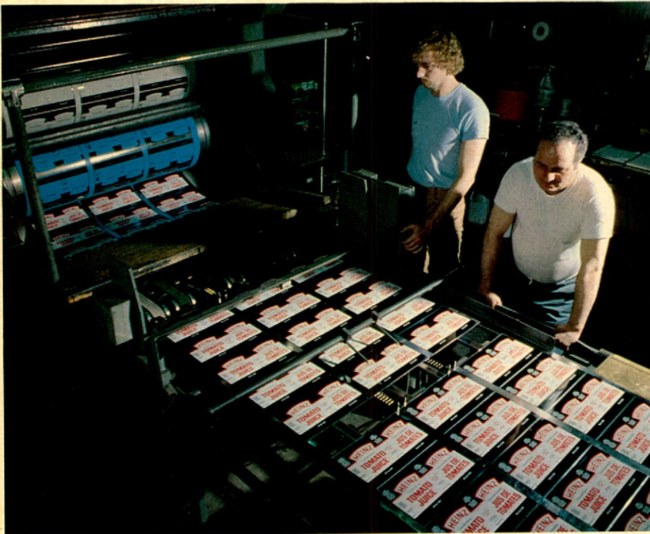
Light-gauge printing press, Metal Decorating Lithographers
