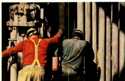
Two roughnecks stack drill pipe while a drill bit is being changed.
