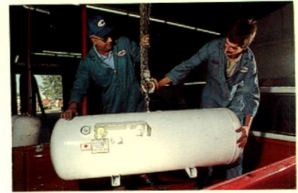
Oil and gas Cigas personnel convert a motor vehicle from gasoline to propane motor fuel at a Cigas conversion centre in Calgary, Alberta.
