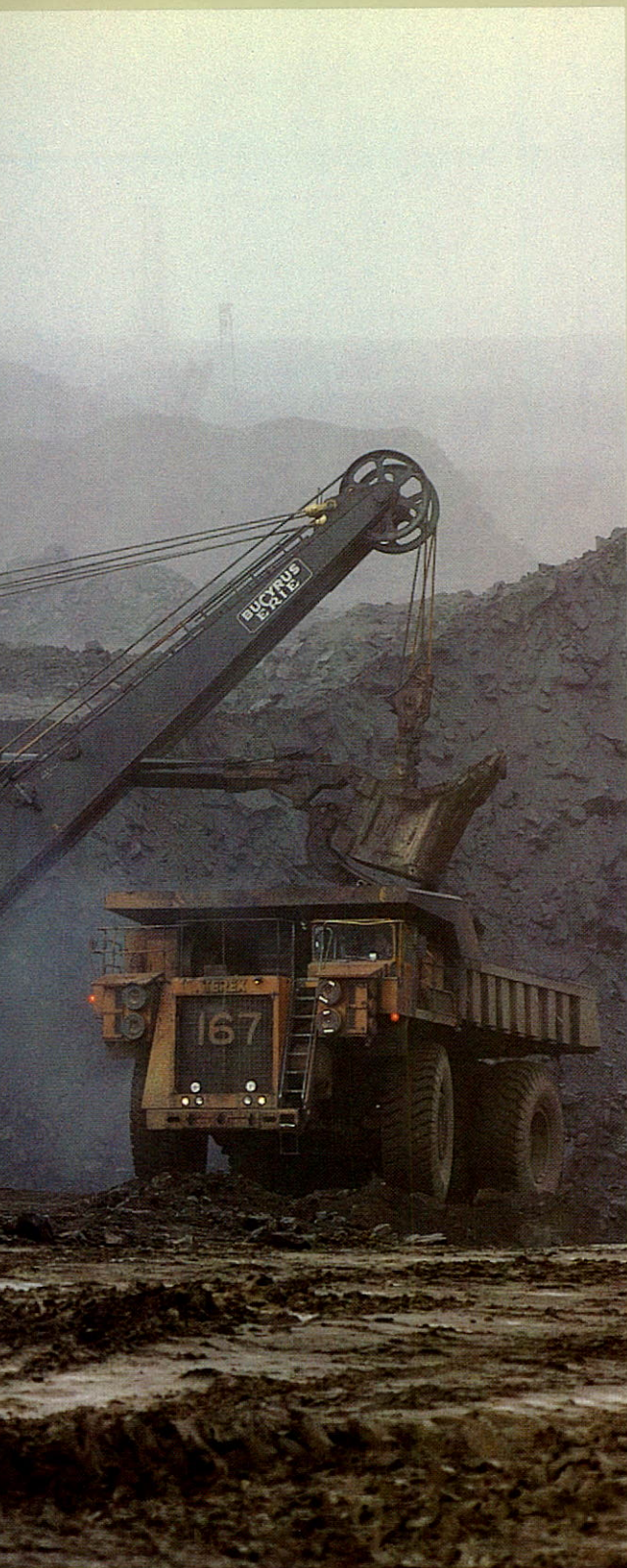
120-ton trucks transport iron ore from the open pit mines at Iron Ore Company of Canada's operations at Labrador City, Newfoundland.
