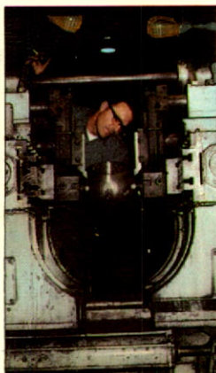
Worker adjusts computer-assisted torches (left) that cut the intricate steel parts used in valve assembly. Machinist (above) examines ball valve. Valve (far right) is coated with epoxy resin to prevent corrosion.
