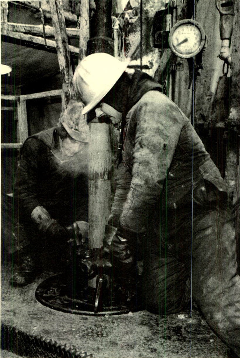
Drilling crew members adjust the drill pipe on one of Husky's exploratory rigs in Alberta.
