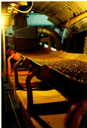
Fuel pellets, made from forest wastes, come off the production line at BioShell's Iroquois Falls plant in Ontario.
