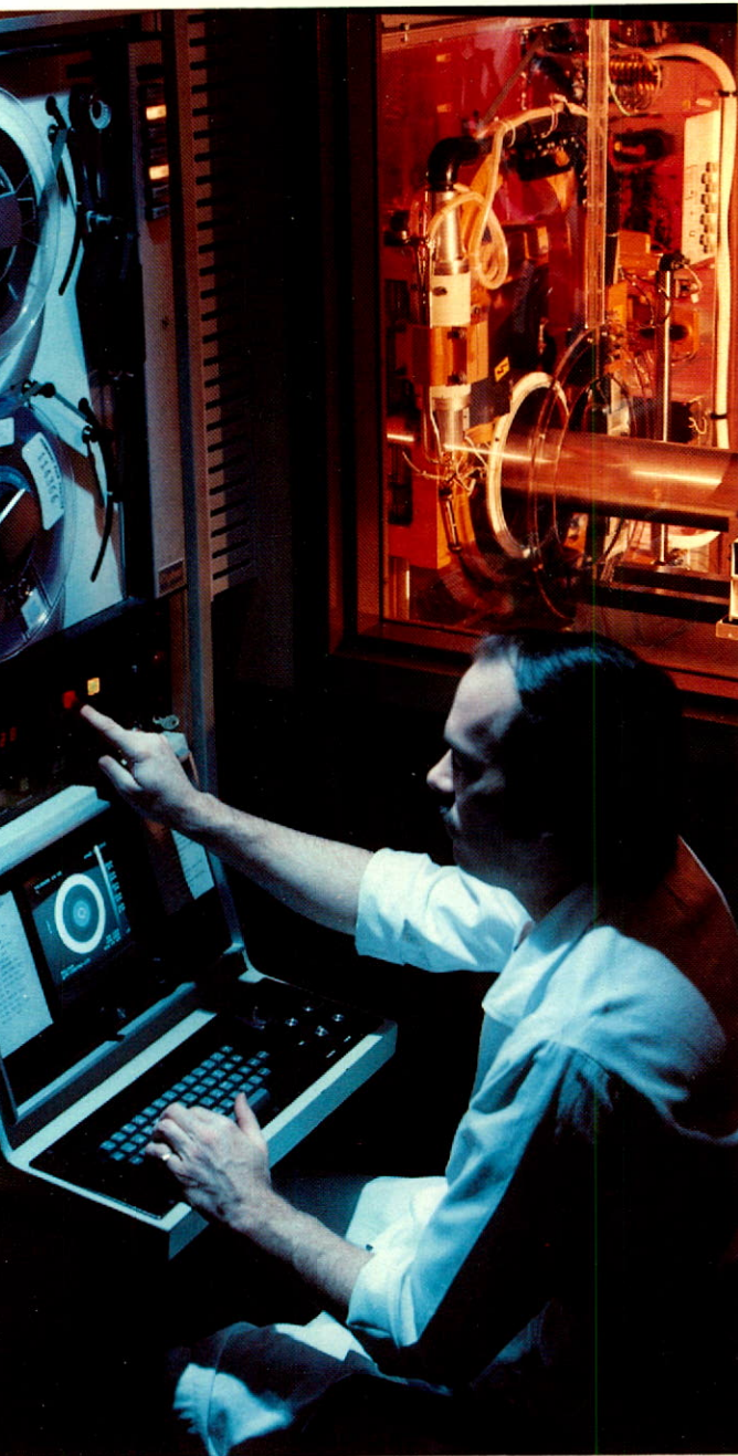
Senior technologist Lyle Serres operates keyboard console of the Calgary Research Centre's computerized tomography scanner (background) to study well core samples for enhanced oil recovery projects, using the same principles as hospital CAT scanners.
