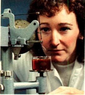
Material technologist Lynn Chandler measures surface tension of a hydrocarbon sample in research laboratory.
