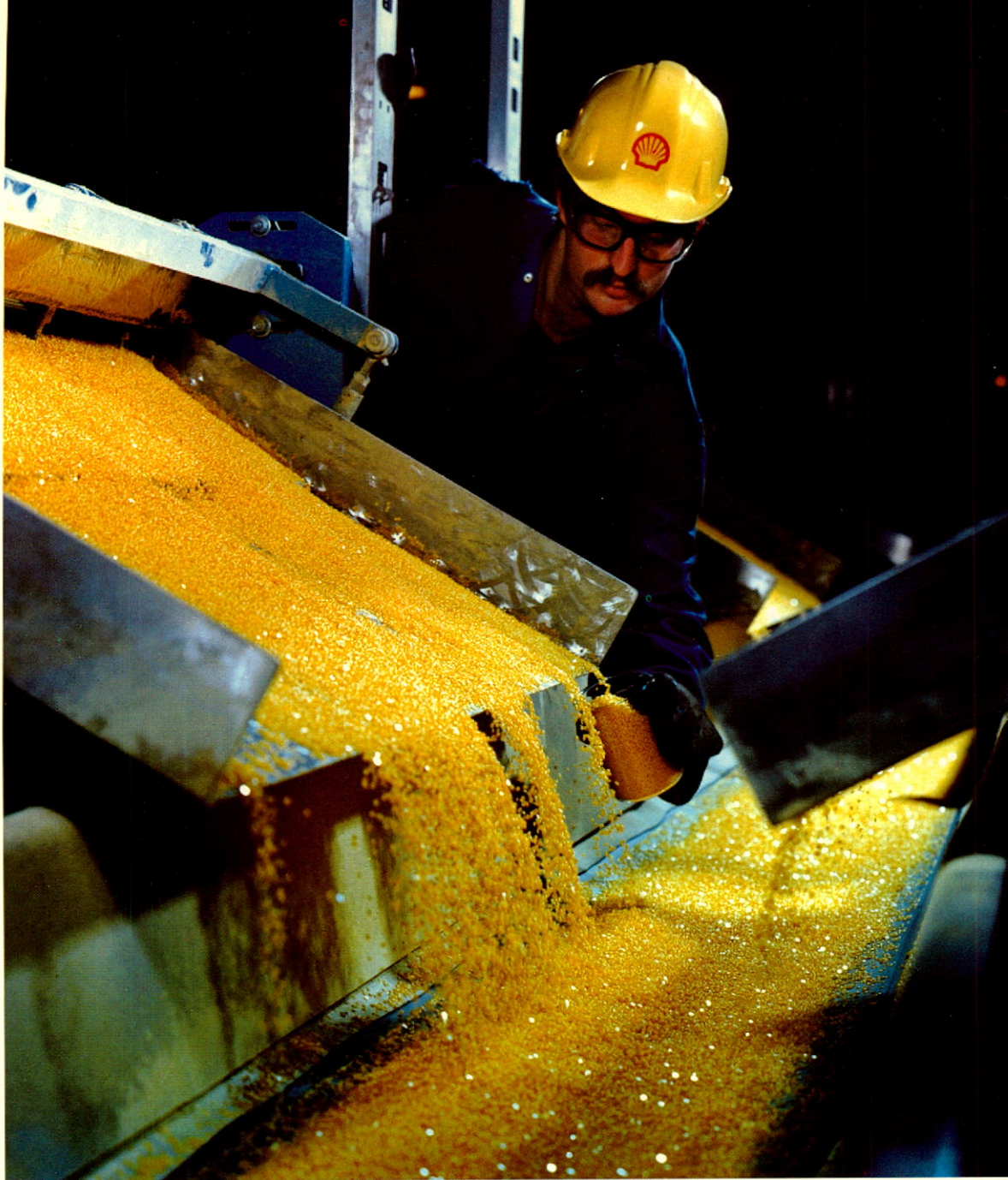
To meet continuing high export demand for sulphur, Shell Canada installed a new pellet-forming unit at its Jumping Pound plant near Calgary. Tim Tivendale monitors the sulphur pellets being produced at the $11 million unit.
