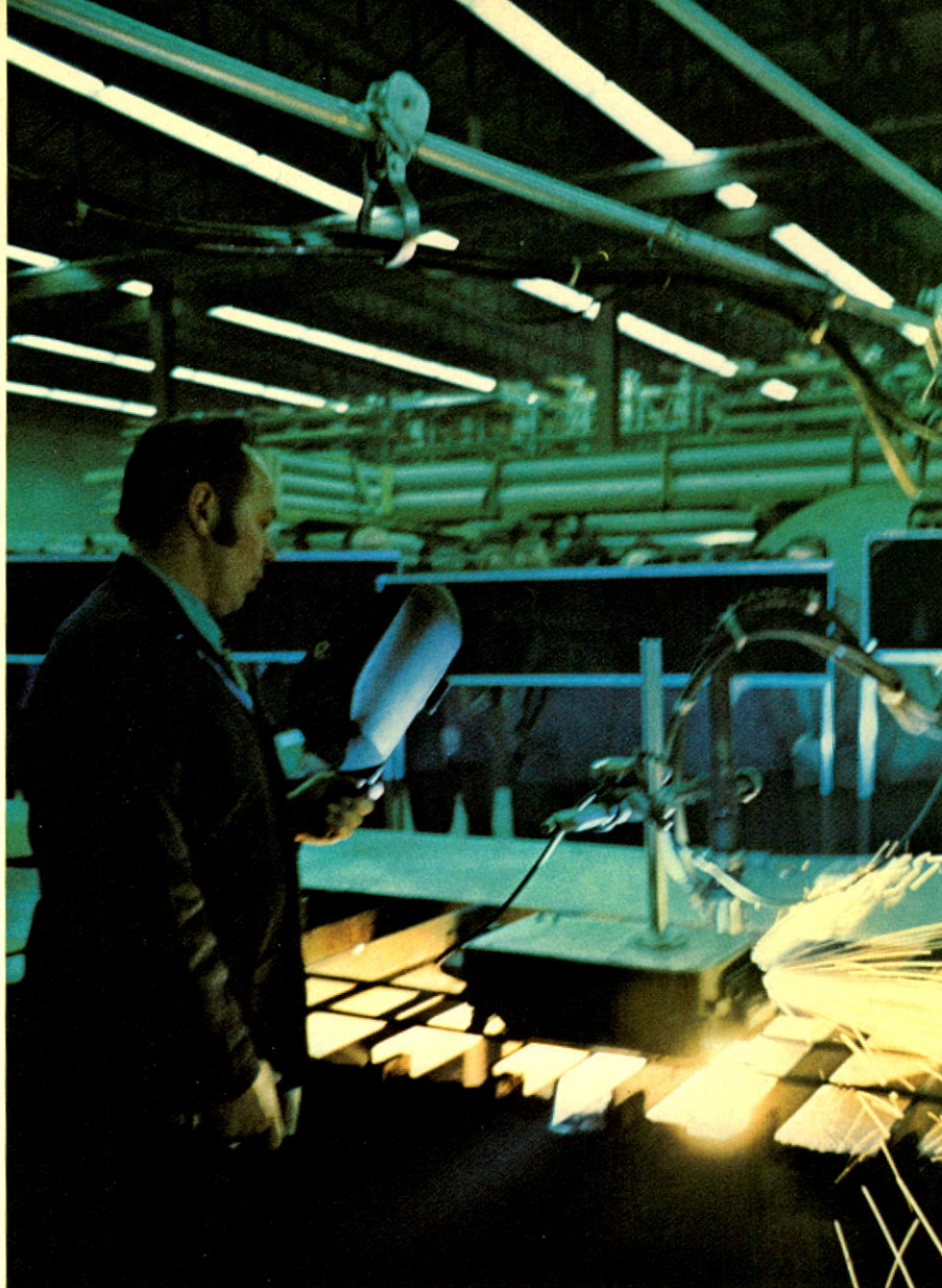
Atlas Alloys, the company's specialty metals distributing arm, opened a new service centre in Montreal with a two-day exhibition showing the latest in modern metals and their applications. Clockwise from top left: Guests check in at registration desk. Dramatic display of ultra high temperature "plasma" cutting guided by operator with remote control. Part of the exhibition area, with Orren S. Leslie, Atlas Steels president (left), and William D. Dobbin, Atlas Alloys general manager, in foreground.
