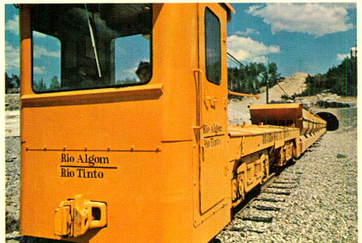
Ore haulage by semi-automatic electric railway from New Quirke uranium mine to the Quirke mill just over a mile apart. The railway went into full operation in early 1969.
