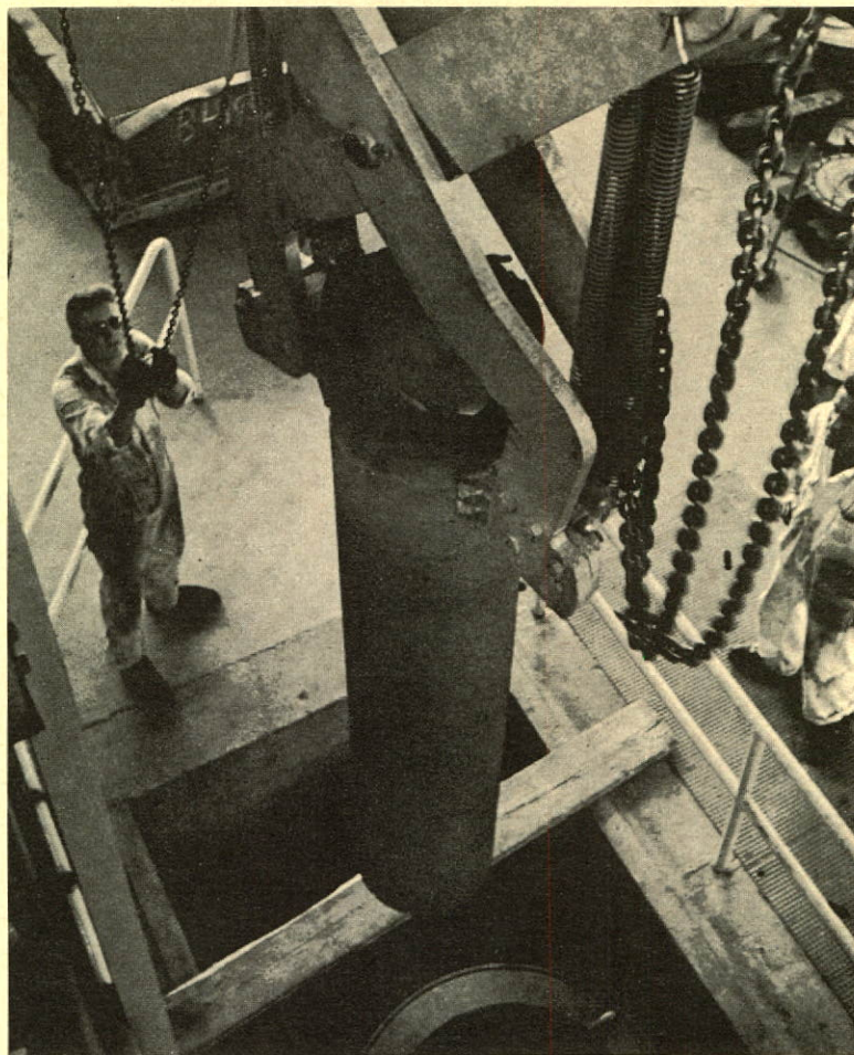
Titanium ingot being removed from remelting furnace. Atlas Titanium division is producing increasing amounts of titanium for a variety of uses but particularly for aero-space application.
