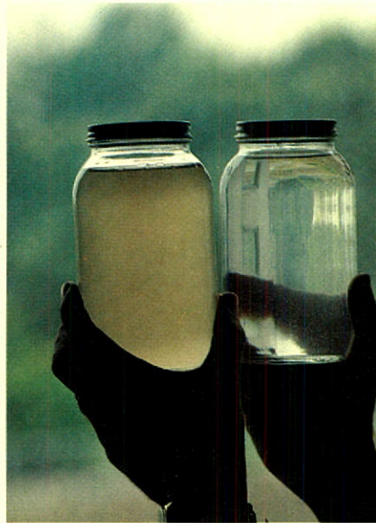
Before and after. Effectiveness of new water quality control system at the Welland plant is evidenced in these two jars of water. The system each day removes mill scale and lubricants from over 6 million gallons of cooling water which is then recycled.
