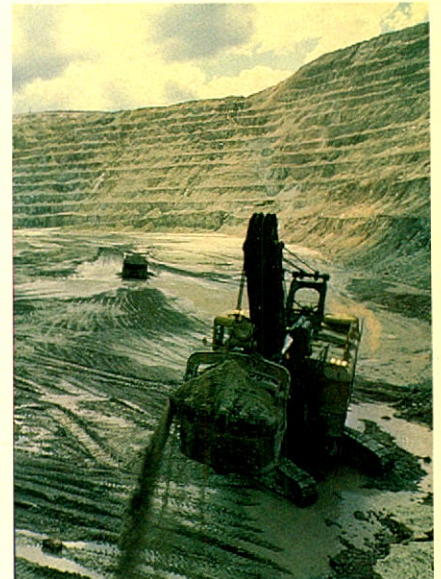
Big bite is taken by 22-yard shovel in the Lornex pit. Haulage volume will increase to 95 million tons of ore and overburden per year as a result of current expansion.
