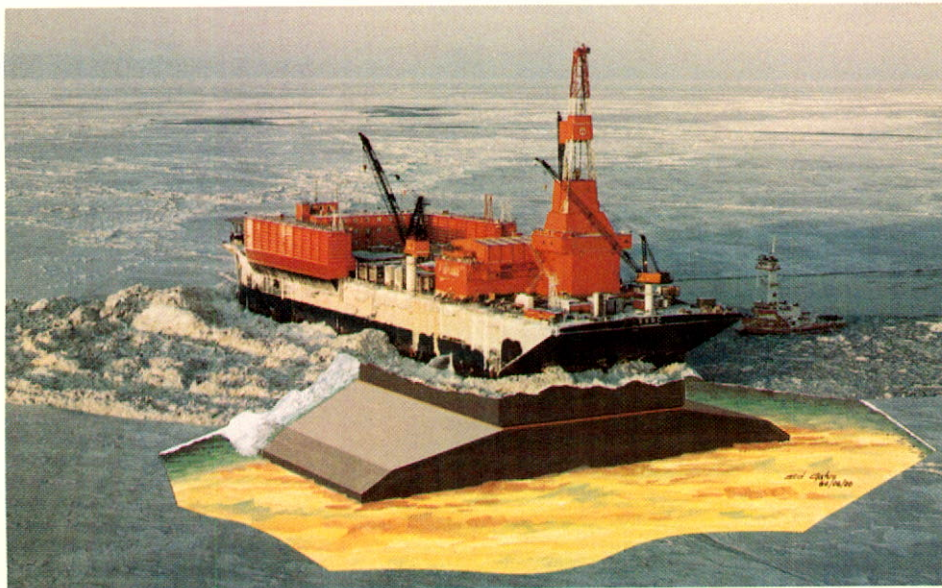
Artist's rendering shows relocatable mat system designed to improve economics of drilling using Dome's SSDC mobile Arctic drilling vessel. Engineering design of the mat system is being developed for a major U.S. oil company.
