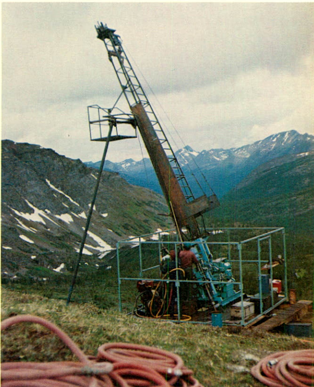
Diamond drilling on a tin prospect in the Yukon Territories
