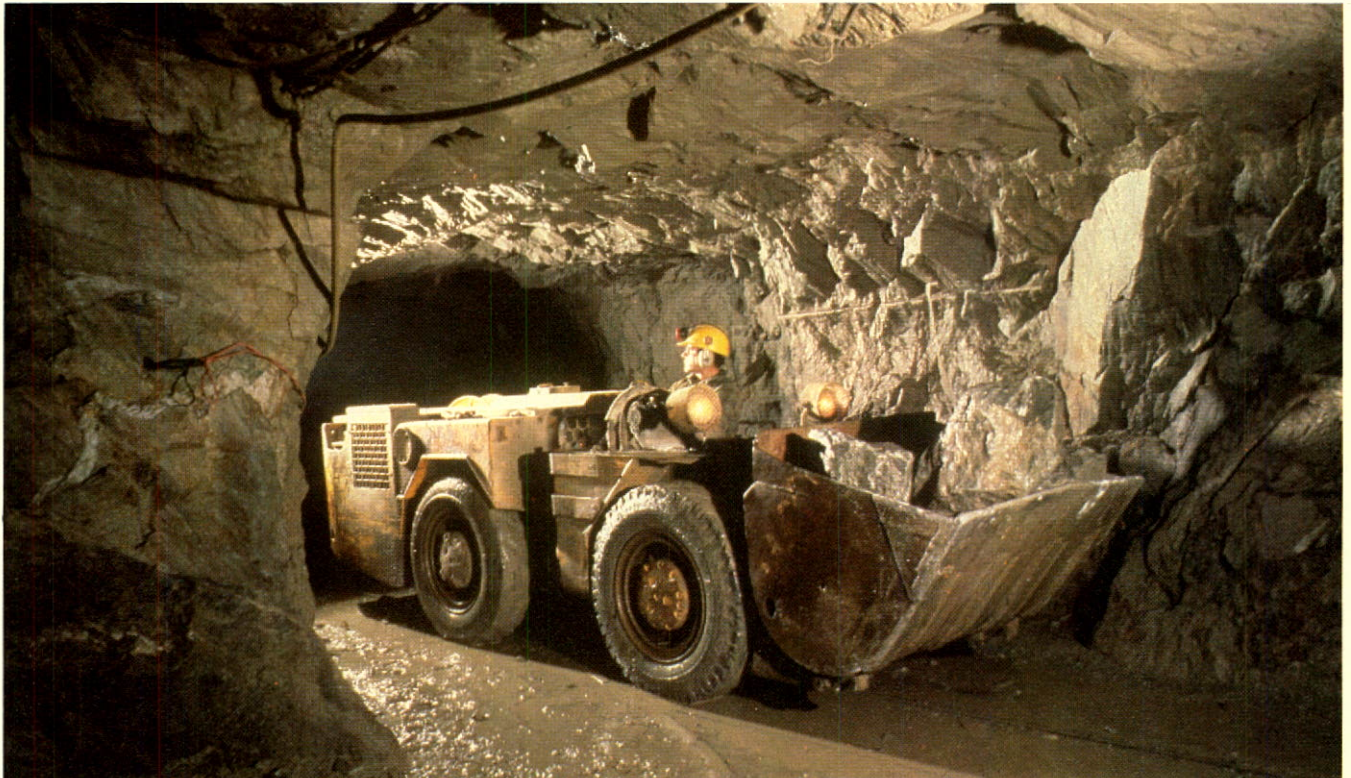
An electric load-haul-dump unit operating underground at the Dome mine.
