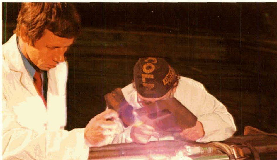
An interchange of new ideas helps each part of Dominion Bridge to learn from the experience of associated groups. Here a process specialist instructs shop personnel in the welding of tubes for large boiler installations.
