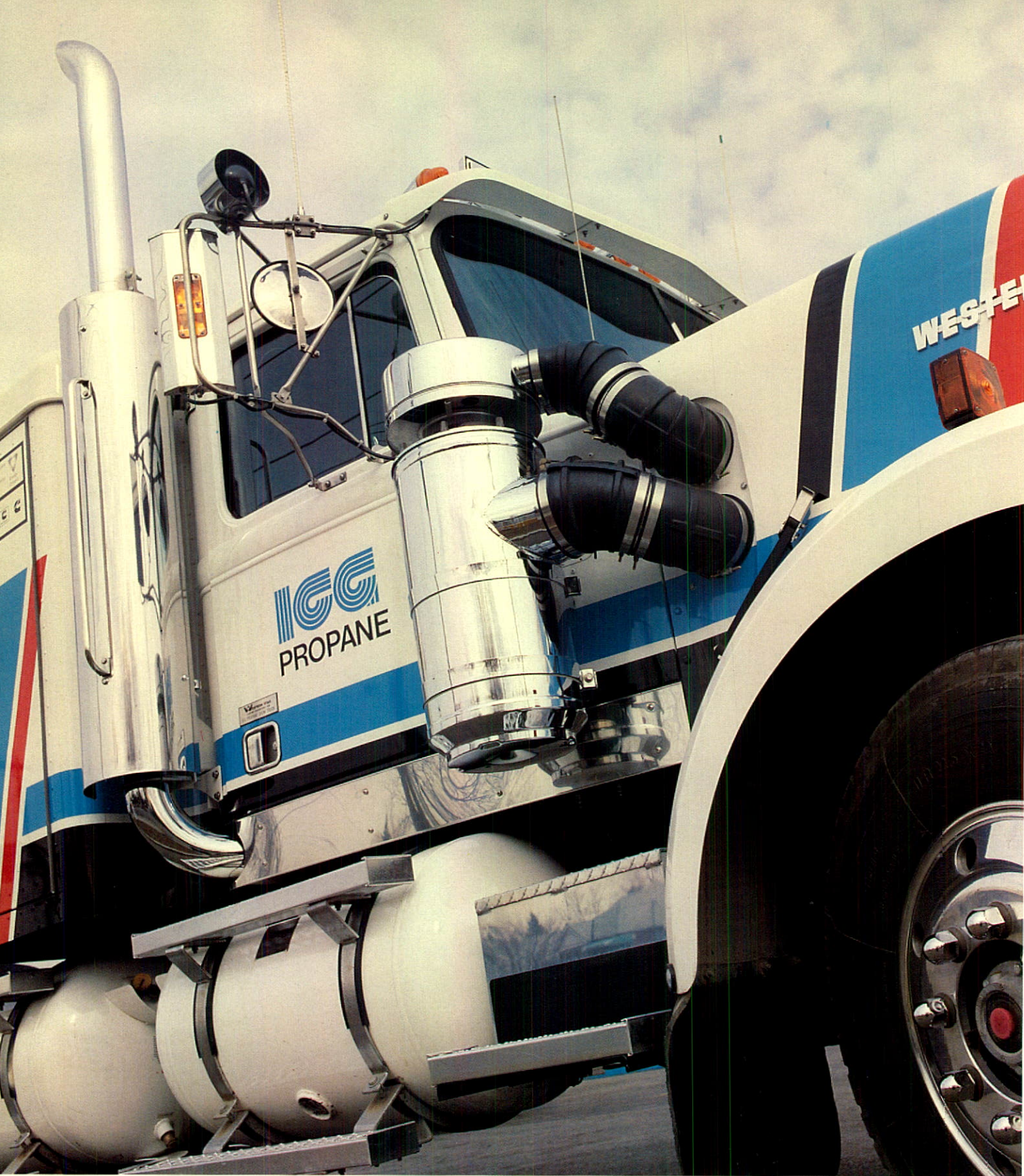
A testing program in co-operation with the Government of Ontario – in which 54,000 km were logged on this prototype vehicle – is proving the advantages of propane over diesel fuel for operators of large trucks. The total potential market is 145,000 Class Eight trucks which would burn approximately 16 billion litres of propane annually.
