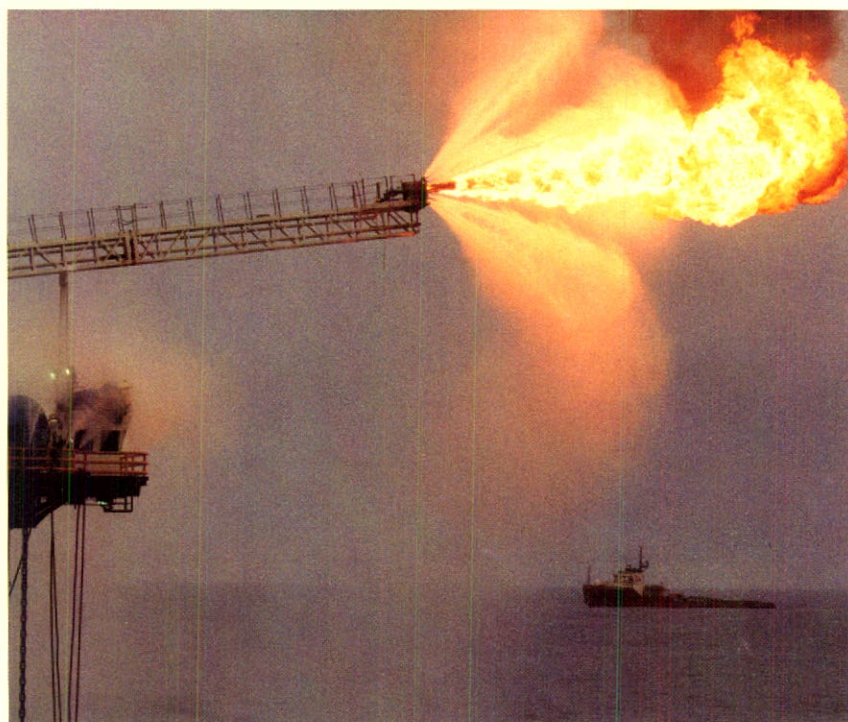
Natural gas is flared at the Terra Nova K-08 oil discovery in the South Hibernia area. Producing from four zones, the well tested in excess of 1700 cubic meters per day.
