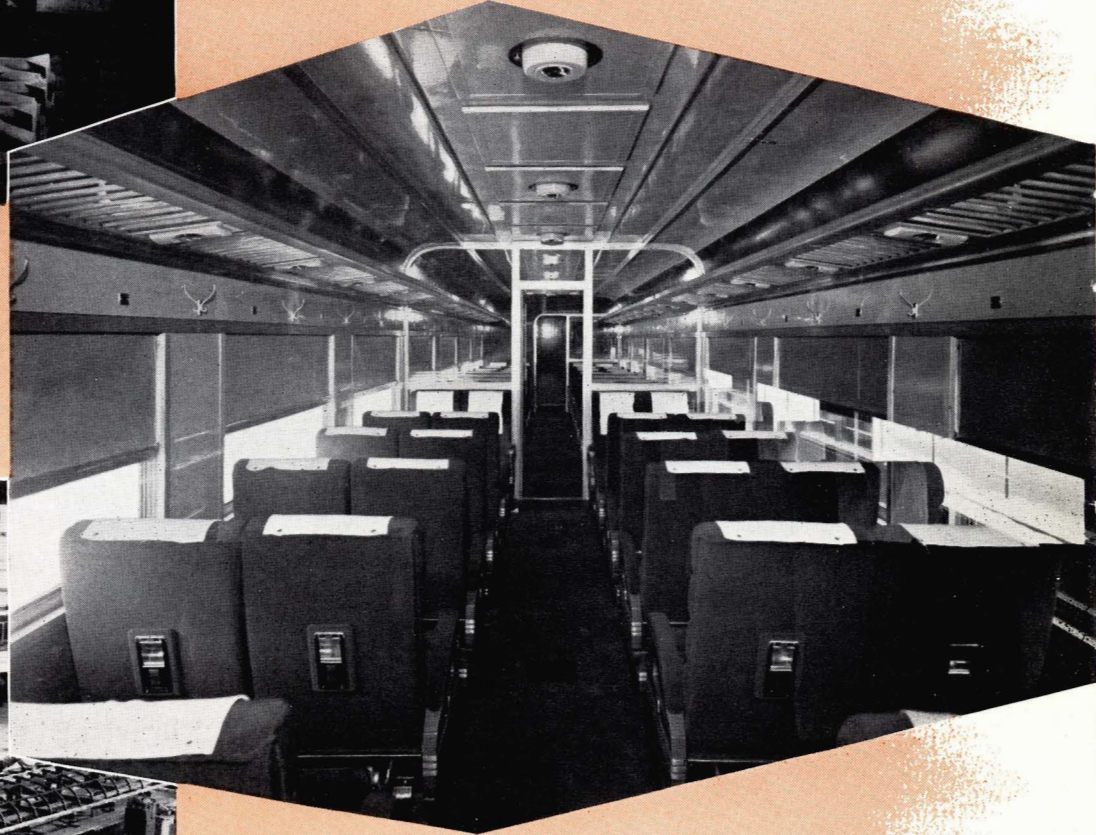
Interior of one of the new all-steel passenger coaches showing the latest type "Sleepy Hollow" adjustable seats; wider windows and improved lighting arrangements.
