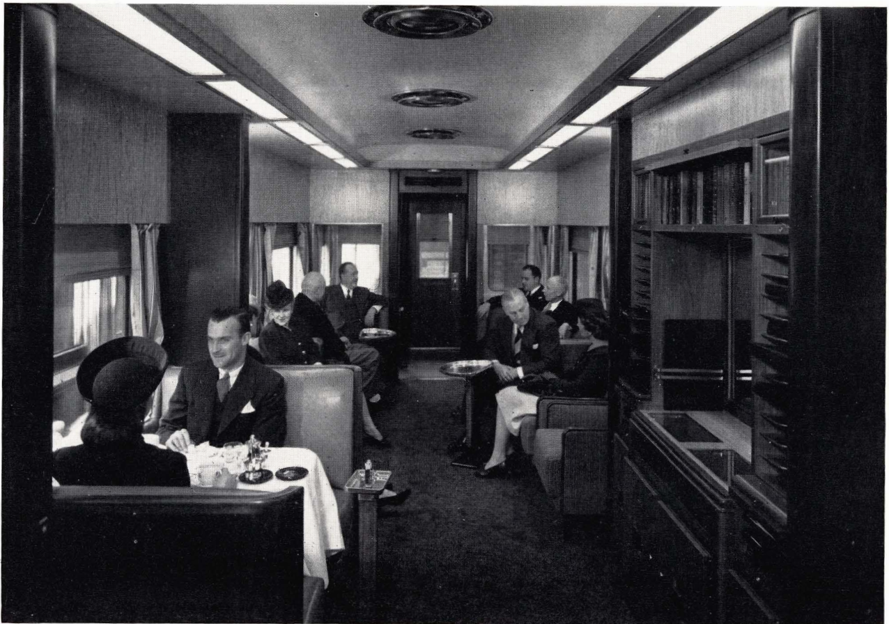
A new type of streamlined bedroom-buffet-lounge car was placed into service during the year. These cars have four single bedrooms which may be converted into suites, a spacious lounge with direct and indirect panelled fluorescent lighting, a solarium and a modern buffet section. They were built in the Company's shops.
