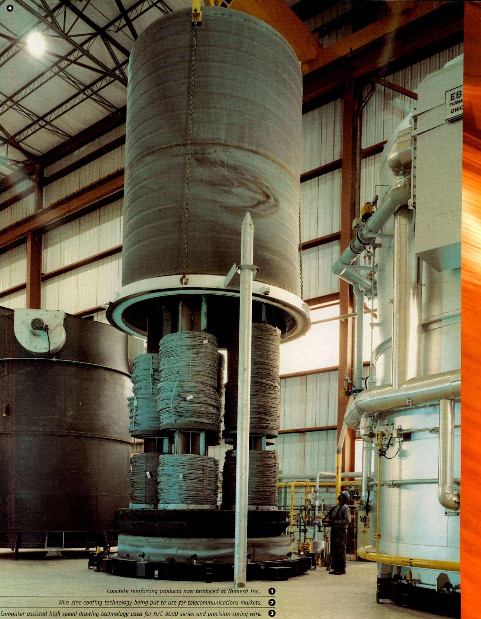
State-of-the-art Ebner annealing technology (protective hydrogen gas atmosphere during cycle). ❹
