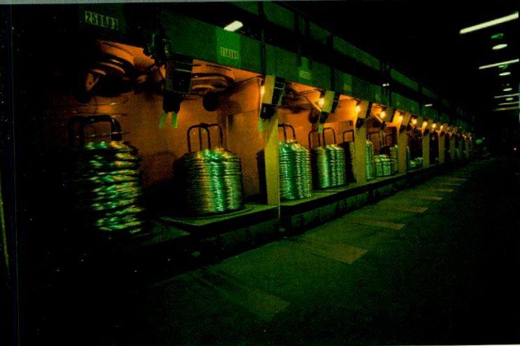
The finished product take-up at the end of the wire galvanizing process.
