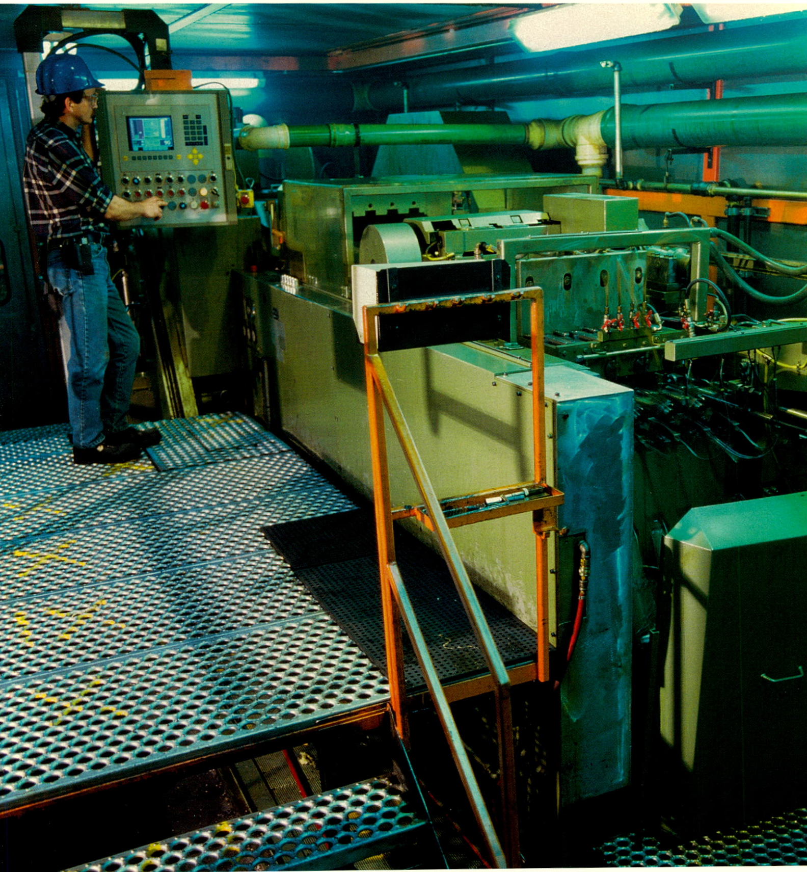
A skilled technician makes adjustments to this modern boltmaker at the Infasco manufacturing complex at Marieville, Québec.
