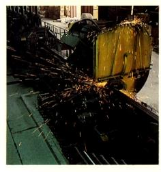
The hollow structural section is cut to specified length by a traveling saw. The saw is directed by a programmable controller that calculates appropriate lengths to customer order.
