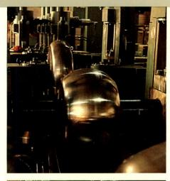
Highly polished forming rolls gradually form flat steel strip into the shape of an arc.
