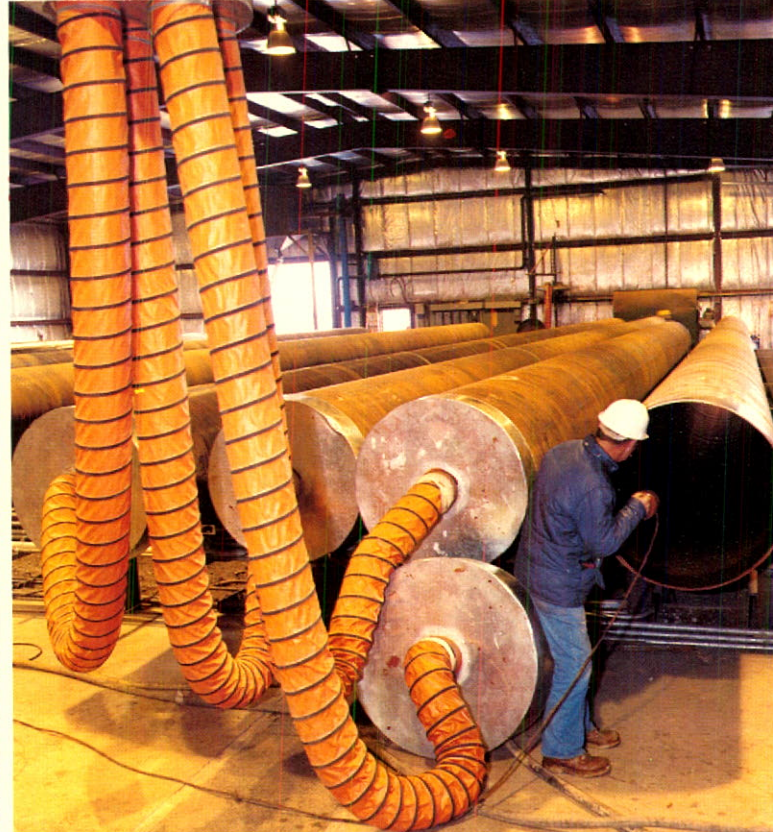
▼ Internal painting of large diameter pipe by Wescan Pipe Protection Ltd.
