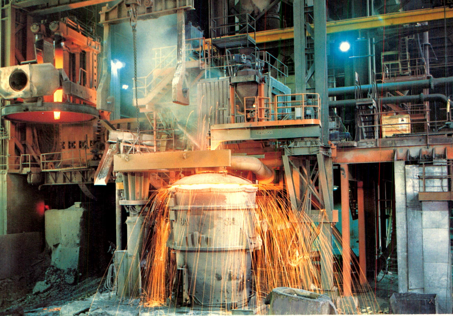
▲ A ladle of molten steel undergoing treatment at the desulphurizing station.
