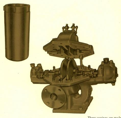
These castings are made of special salt-water resistant bronze. Upper left, a spun cast stern tube bushing used in the steering mechanism of ships. The other is a marine refrigeration pump used on food carrying ships.
