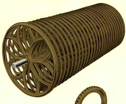
In the production of pulp and paper, the large "spider" castings, illustrated above, are used to make up cylinder moulds.
