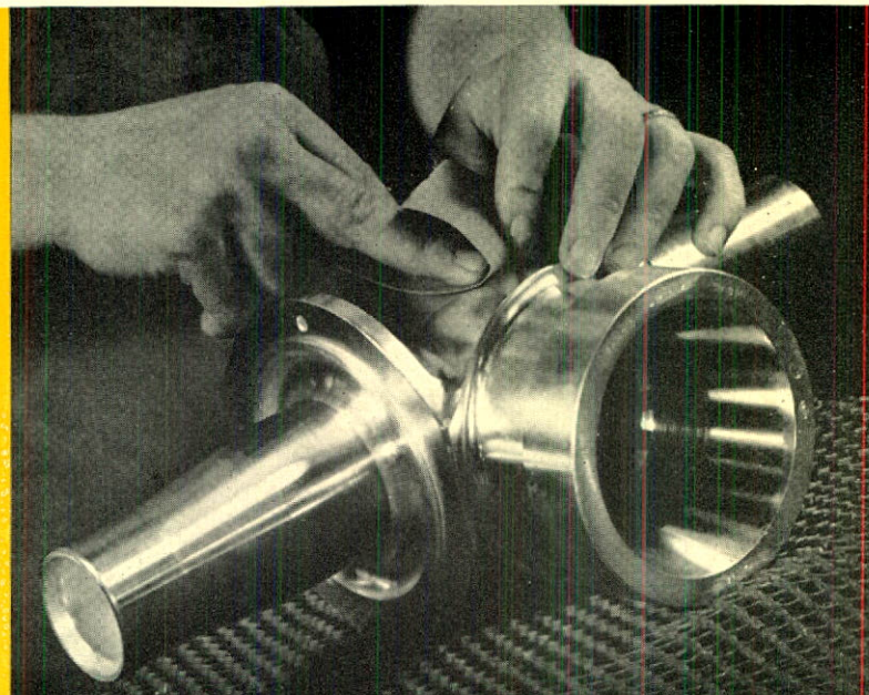
Polishing a Hamilton Standard Spider for the propeller of a Harvard Trainer.
