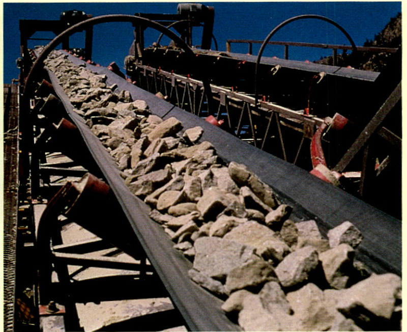
Industrial fabrics are used in the manufacture of conveyor belts such as those found in the mining industry and in quarries.
