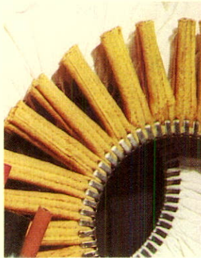
Industrial fabrics are engineered to meet the requirements of many manufacturing and process industries. This buffing wheel is used mainly for polishing metals.
