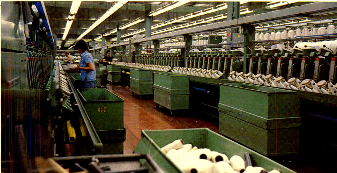
Modern winding facilities automatically and efficiently transfer yarn to large packages for the next process.
