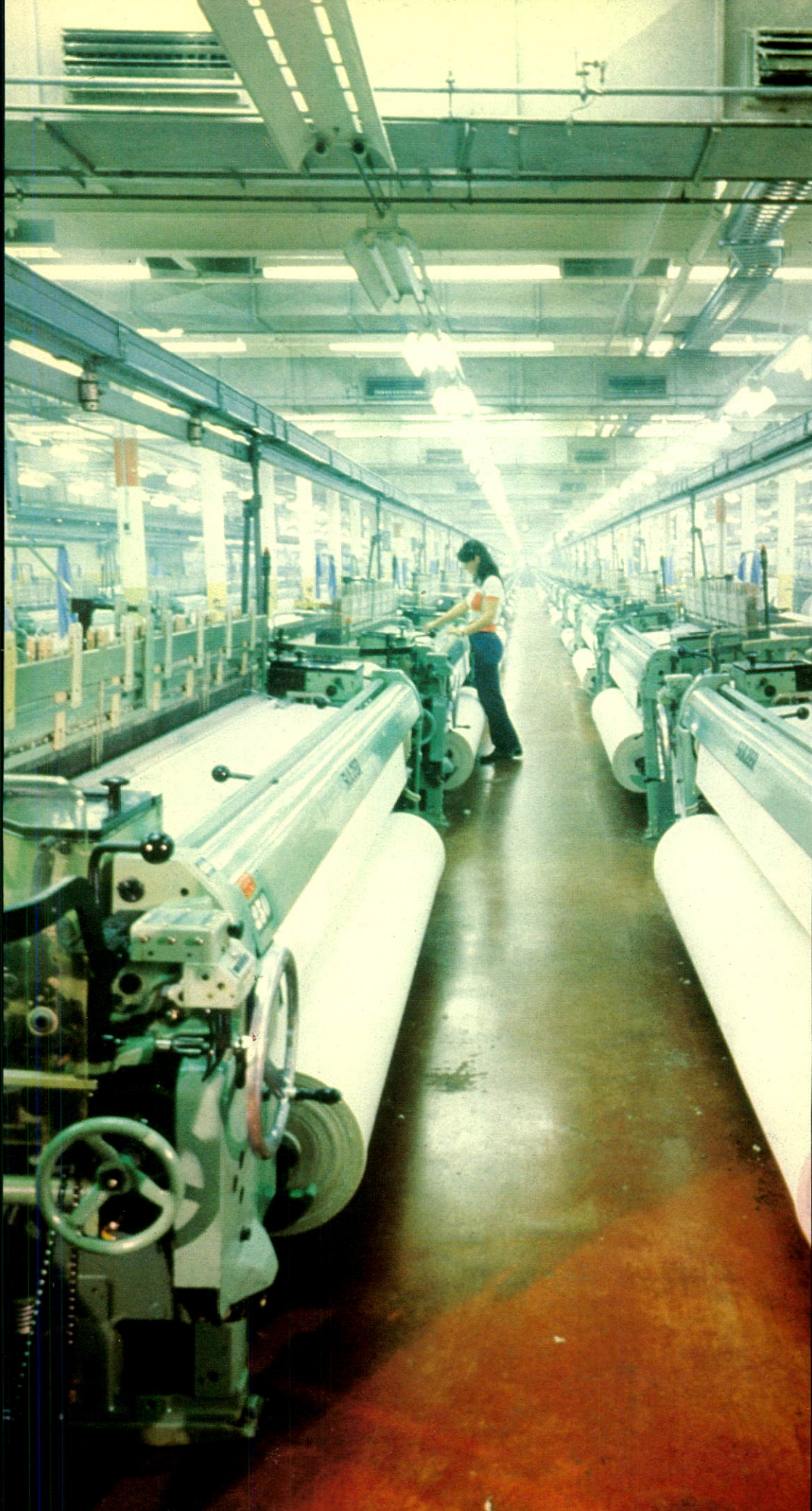
Projectile weaving machines produce fabric at double the rate of conventional looms.
