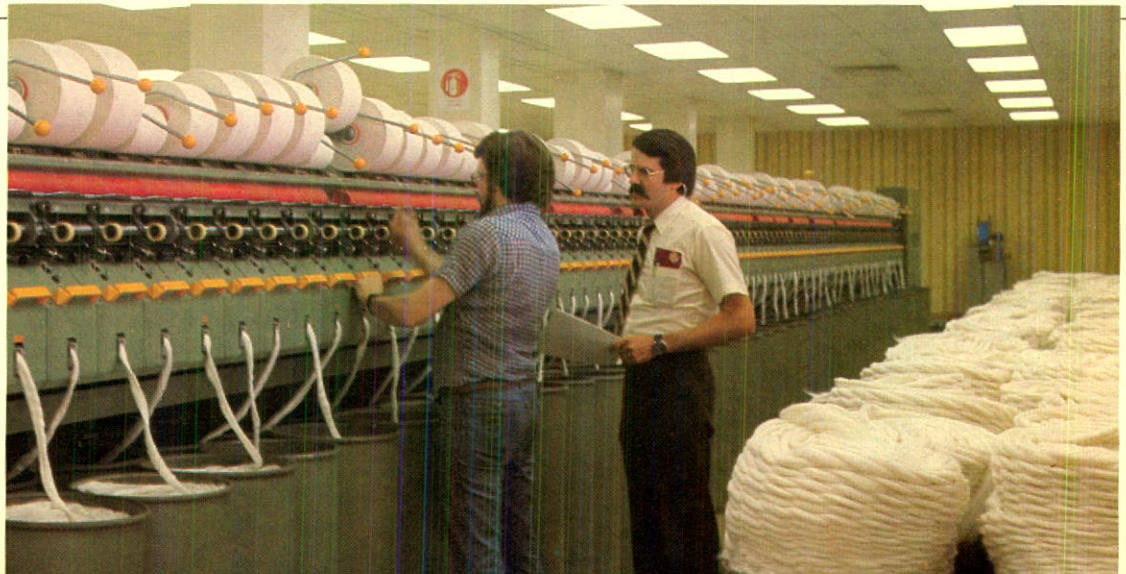
Open-end spinning replaces a number of manufacturing processes and produces better quality yarn at rates ranging from 3 to 9 times that of ring spinning.
