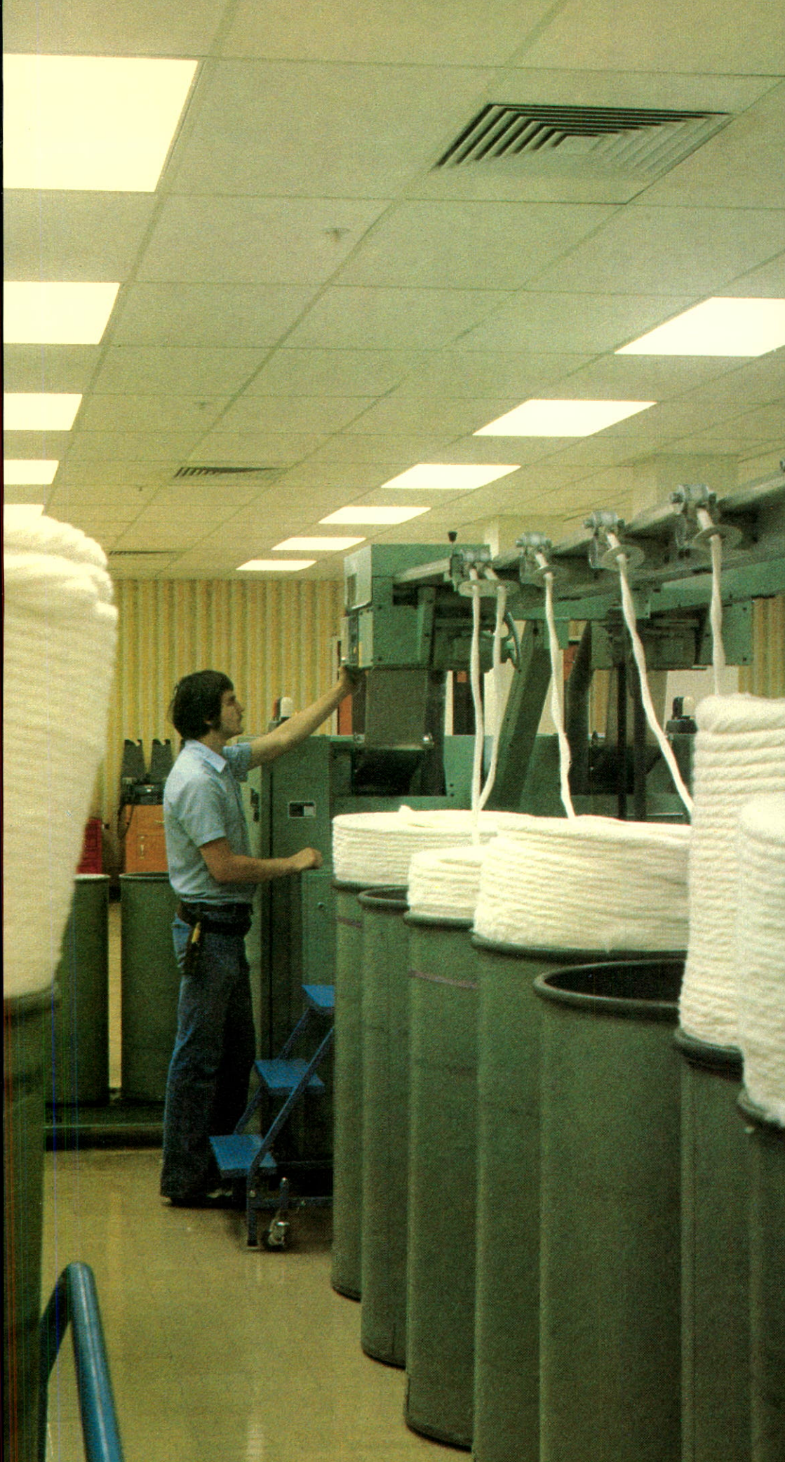
High speed drawing frames produce a more even and superior product at double the conventional rate.
